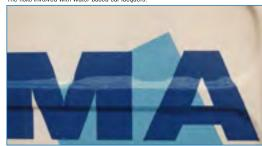
Due to the silicone content in modern car lacquers the adhesion of film can be far from optimal. Film under tension (especially in recesses) is bound to come loose and ultimately be returned for repair or renewal.
