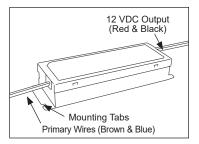
3. **Power Supply:** Identify primary wires, secondary wires, and location of mounting tabs.
