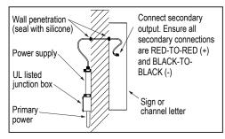
7. Make secondary connections: Secondary class 2 cables do not require conduit per NEC 2008 Articles 725.121 through 725.130. Seal all wall penetrations with silicone to avoid water damage.
