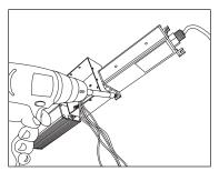
5. Mount Power Supplies: Units may be mounted in any orientation using mounting tabs.
