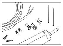
2. Supplies required: Junction box, #8 or #10 pan head screws, UL Listed PLTC cable, electrical wire connectors, ½ in (13 mm) locknuts, silicone
