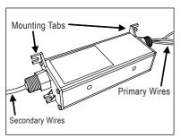
3. Power Supply: Identify primary wires, secondary wires, and location of mounting tabs.
