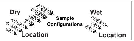
4. Configure Power Supplies: Secure power supplies to junction box using ½ in (13 mm) locknuts. Power supplies may be joined together in a wide array of configurations. For wet locations use a junction box that is UL Listed for wet locations. For dry locations, use any UL Listed junction box.
