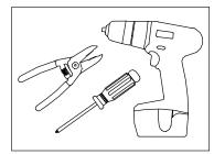
1. **Tools required:** Wire strippers, drill, and screwdriver.
