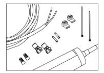
Supplies required: Electrical enclosure for power supply, M4 pan head screws, PLTC cable, silicone, 3M<sup>™</sup> Scotchlok<sup>™</sup> connectors.
