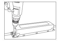
4. **Mount Power Supplies:** Use mounting tab in corner to secure power supply.
