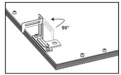
Insert fixture in T-Bar grid, and bend hook tabs over T-Bar to capture rails. Proceed to Finishing Installation section on page 4.
