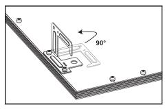
1. Bend metal tabs on back of fixture, 90° to form "L" hook.
