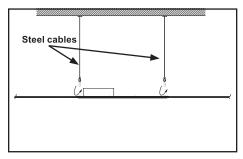
1. Ensure existing steel cables are secure, and align fixture with steel cables.
