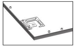
2. Bend metal tabs on back of fixture 90° to a standing position.
