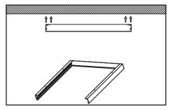
Install Mounting Box on ceiling. NOTE: For part numbers FP10-6060-4040(X), FP10-6262-4040(X), FP10-3012-4040(X), and FP10-6012-5040(X), connect power supply and attach, according to local regulations, before proceeding to next step.
