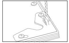
2. Secure all four corners of fixture to steel cables. Proceed to **Finishing Installation** section on page 4.
