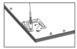
Secure all four metal tabs, on corners of fixture, to steel cables, and attach to ceiling structure per local code. Proceed to Finishing Installation section on page 4.
