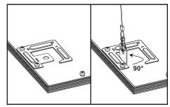
Bend metal tabs on back of fixture 90° to a standing position. Secure all four corners of fixture to steel cables with mounting clips, and attach to ceiling structure per local code. Proceed to Finishing Installation section on page 4.
