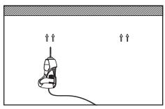
1. Prepare ceiling for steel cable installation by installing anchors into ceiling.
