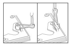
Secure all four corners of fixture to steel cables with mounting clips. Proceed to Finishing Installation section on page 4.
