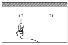
Prepare ceiling for steel cable installation by installing anchors into ceiling.
