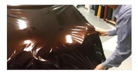
Set the heat gun to the maximum and warm the film surface by circulating movements of the heat gun.
