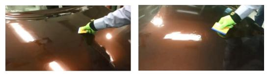
Apply the film with your finger in concave parts where necessary and continue squeegeeing.
