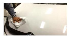
Note: Do not use isopropyl alcohol as this can affect the adhesion of the film. Other solvents than 3M<sup>™</sup> Surface Preparation System may affect the adhering properties of the film, too.
