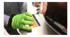
Apply the film lengthwise from the center outwards with overlapping strokes and ensure that the squeegee is in constant contact with the film. 3M Controltac technology ensures that the film is flexible on the surface and adheres only when pressure is applied, whilst 3M Comply technology allows air to be easy removed without causing bubbles.
