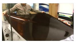
Span the film with low tension on the substrate to remove larger wrinkles but do not stretch the film at the edges.
