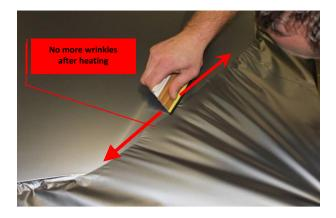
Application on The film is designed for application on flat and simply curved surfaces. On recesses and deep channels it is recommended to apply the film with inlays. Please refer to the Instruction Bulletin Inlay Method for details.
