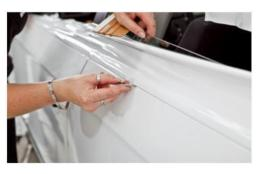
Cut the film at an overlap of approx. 2 mm on the gasket and apply the film with the squeegee underneath the gasket. For cutting the use of Knifeless Tape is recommended.
