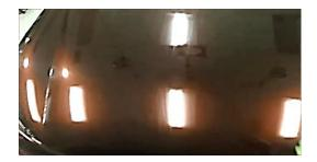
Check film application on air entrapment by re-heating. Remove air bubbles between the film and the substrate with an air release tool and press the film again onto the substrate.
