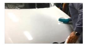
After cleaning make sure that the substrate, edges and seams are completely dry. Film adheres poorly even to a properly cleaned substrate if there is any remaining liquid on the substrate, edges or seams.
