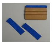
1080 requires high squeegee pressure to avoid air entrapment between film and substrate. Therefore the use of 3M<sup>™</sup> PA-1 Gold Squeegee with thin and soft sleeve (microfibre sleeve) is recommended. Wetting of sleeves helps to avoid scratches on film surface during application.
