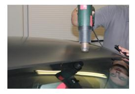
1080 Carbon Fiber and Brushed may tear at higher temperatures if being slightly stretched. Therefore, heating temperatures for these films should not be higher than +40°C to +50°C.
