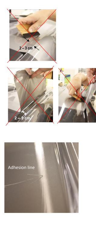
ApplicationIn bridging situations, stop applying the film at least 10 cm before the edge in order to reduce tension of the<br/>film. Then lift the film slightly and continue tension-free squeegeeing to the edge.RecommendationIt is recommended to do the application in one step without interruption.
