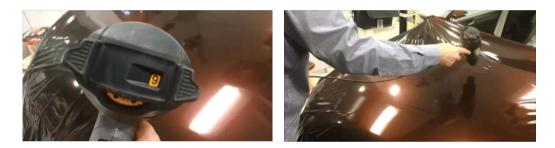
The film surface should reach a temperature of +30°C to +40°C.
