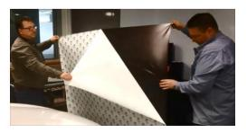
Application on Flat Place the film without tension on the substrate. Controltac™ adhesive technology provides easy sliding of the Surface film.
