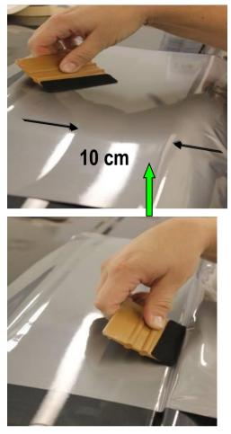
It is very important NOT to squeegee the film directly after heating. Let the film cool down for a few seconds after heating, then firmly squeegee without stretching the film. Stretching at the edges might cause shrinkage of the film and color fading.
