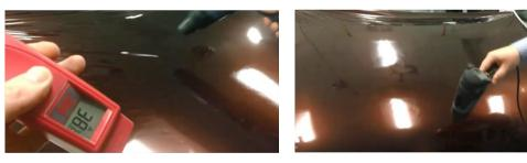
By heating the film and letting it cool down, wrinkles disappear and the film will conform to the surface so that squeegeeing will be possible without repositioning of the film.
