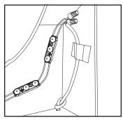
Connect power supply to first module on string: See power supply install guide for more information regarding power supply installation. NOTE: For SloanLED Prism Nano, to avoid significant line loss, do not use more than 6.56 ft (2.0 m) in series (see diagram on page 2 of this install guide).
