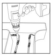
Fasteners: If desired, modules can be secured with #6 (3.5 mm) pan head sheet metal screws or 1/8 in (3 mm) aluminum rivets.
