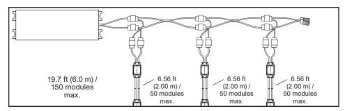
**NOTE:** For SloanLED Prism Nano, to avoid significant line loss, do not use more than 6.56 ft (2.0 m) / 50 modules in series.
