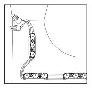
Cap all unused wires: The strand of modules should not be looped to create a closed circuit.
