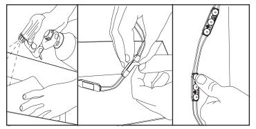
4. Peel and stick: Clean inside sign with rubbing alcohol and allow to dry. Using predetermined layout and LED placement from Step 3, remove tape backing and stick modules into place. Ensure modules are firmly attached. NOTE: If installing SloanLED Prism Nano, and installing in a narrow channel, tape may be unnecessary. Other means of securing strip (sealant, vinyl, etc.) are also acceptable.
