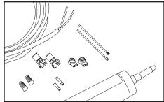
Supplies required: PLTC cable, wire nuts, IDC connectors or butt splices with appropriate safety agency markings, and cable ties. <u>Optional</u>: Screws and silicone.
