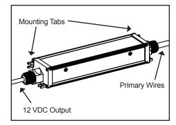
3. Power Supply: Identify primary wires, secondary wires and location of mounting tabs.
