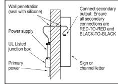
7. Make Secondary Connections: Secondary class 2 cables do not require conduit per NEC 2008 Articles 725.121 through 725.130. Seal all wall penetrations with silicone to avoid water damage.
