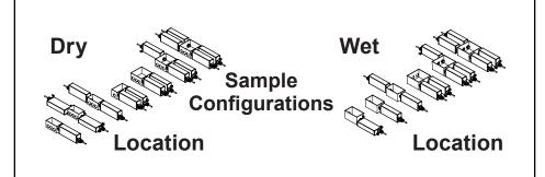
**4. Configure Power Supplies:** Secure power supplies to junction box using ½" locknuts. Power supplies may be joined together in a wide array of configurations. For wet locations use a UL listed for wet locations junction box. For dry locations use any UL listed junction box.
