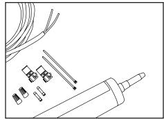
2. Supplies required: Junction box, #8 or #10 pan head screws, UL listed PLTC cable, electrical wire connectors, 1/2" locknuts, silicone.
