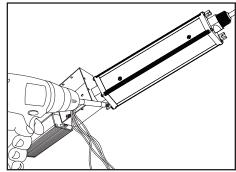
5. Mount Power Supplies: Units may be mounted in any orientation using mounting tabs.
