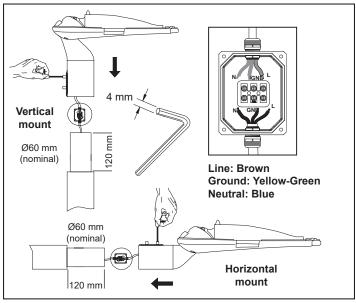
4. Wire and attach base to pole or tenon.
