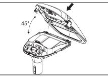
5. Attach body to base hinges at a 45° angle, and close Small fixture. Power is automatically reconnected when Small fixture is shut and power disconnect socket is fully closed. Reconnect flat, three-pole connector in Medium fixture, and close Medium fixture.
