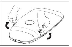
Unlock clamps on sides of luminaire. NOTE: When Small fixture is hinged open, power is automatically disconnected from fixture body.
