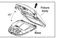
Fixture body can be removed from base by tilting it to 45°, disconnecting primary power at flat, three-pole connector in Medium body fixtures, and pulling it off of hinges.
