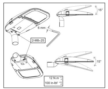
3. Install slipfitter to base in desired position. **NOTE:** Installing slipfitter is easier if base is removed from fixture body.
