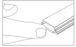
5. **Push PCB back into extrusion:** After Humiseal has dried for at least 7 minutes, press the circuit board as far into the tube as it will go.
