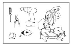
**Tools:** *Required:* Wire strippers, measuring tape, miter saw (for custom length field cuts), multimeter. *Optional:* Cordless drill, drill bits, #2 Phillips driver bits, chalk line.
