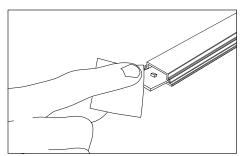
3. Deburr LED board and extrusion: Gently pull LED board out of extrusion about ¼ in (6 mm). Deburr cut-end of LED Board and SlimLINER extrusion with enclosed sandpaper. Make sure to remove all debris from LED board and extrusion.
