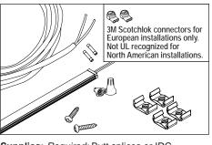
Supplies: Required: Butt splices or IDC connectors, wire nuts, IPS Weld-On® #16 Solvent Cement, and UL listed wet location, sunlight resistant PLTC cable. Optional: Mounting clips (P/N 401203), #6 Pan Head Phillips screws, appropriate thread anchor for the mounting surface. NOTE: 3M<sup>™</sup> Scotchlok<sup>™</sup> connectors for European installations only.
