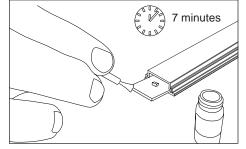
Seal end of LED board with conformal coat: Brush Humiseal 1B73 conformal coat onto cut edge of LED board to seal from moisture. Allow to dry for 7 minutes. Do not apply conformal coat to cut edge of extrusion or end cap.
