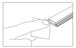
Clean extrusion: Ensure end of extrusion is clean and free of any foreign material. If any Humiseal adhered to the extrusion, gently sand off. Avoid sanding the edge of the LED board.
