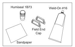
1. **Gather materials:** Sandpaper, Weld-On #16, Humiseal 1B73 conformal coat (for sealing edge of LED board), and acrylic field end cap.
