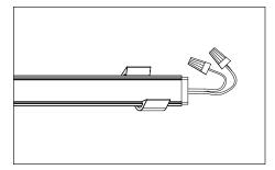
Connections: Sections may be connected in series or parallel. The string of SlimLINER luminaires should not be connected to create a closed circuit. Cap all unused, exposed wire ends.
