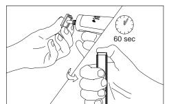
7. **Cap custom cut lengths:** Clean any debris from cut end and ensure that any exposed wires are not in contact with each other (trim wires if necessary). Apply IPS Weld-On #16 to entire rim of SlimLINER field end cap and bond to the cut end of SlimLINER segment. Apply pressure to end cap for 60 seconds to ensure a strong bond. **NOTE:** After cutting a custom length, any piece with black and red wires protruding from original end cap will still light.
