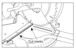
Cutting custom lengths: Each SlimLINER can be cut in the field—for two (2) usable sides—in approximate 5 ½ in (140 mm) increments. If a custom length is required, use a power miter saw to make a clean, straight cut on the black cut line. NOTE: Perpendicular cuts ONLY. Set miter saw to 0°. No angled cuts. After cutting, each piece will still light if connected to power.
