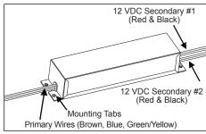
3. Power Supply: Identify primary wires, secondary wires, and location of mounting tabs.
