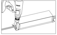
4. Mount Power Supplies: Use mounting tab in corners to secure power supply.
